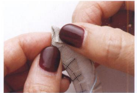
12 Fold the seam allowance at the end in and cut off the dog ear to lessen the amount of fabric to turn under. Fold the side seam over neatly, being careful to keep the edges from showing on the right side.
